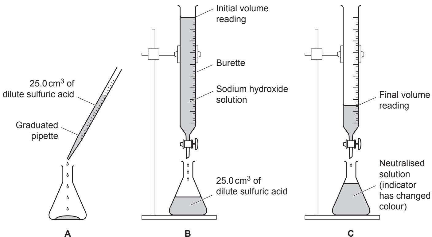
The student adds sodium hydroxide solution from the burette to the sulfuric acid until the indicator changes colour.
