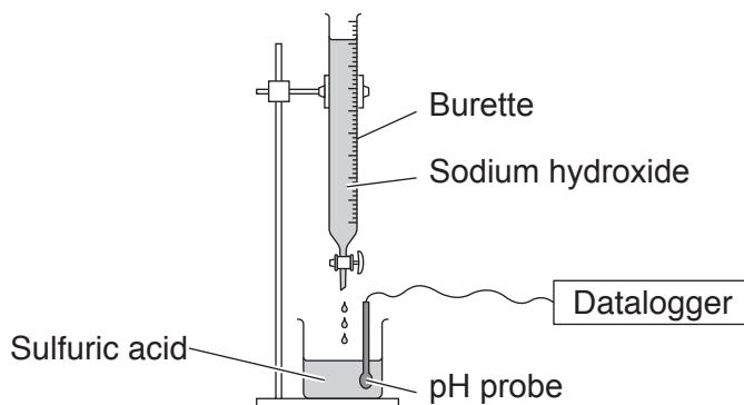
Sodium hydroxide solution is slowly added to the beaker of dilute sulfuric acid.
