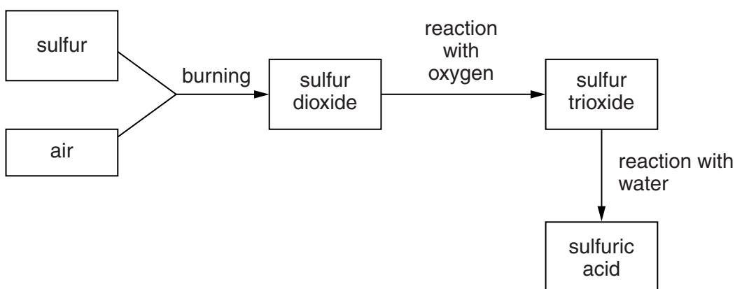
In the process, sulfur dioxide reacts with oxygen to make sulfur trioxide.
