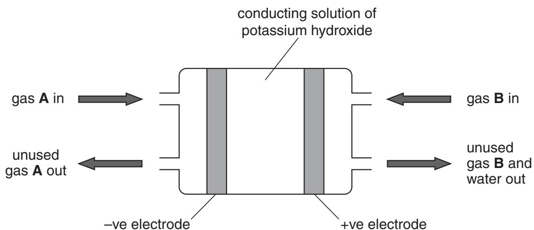
A fuel cell produces electrical energy.
