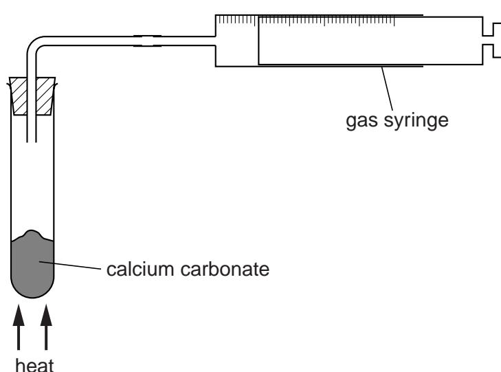
The carbon dioxide made is collected in a gas syringe.
