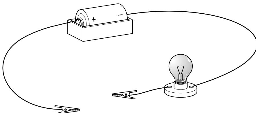
(a) The lamp glows when she puts a piece of copper into the circuit between the clips.
