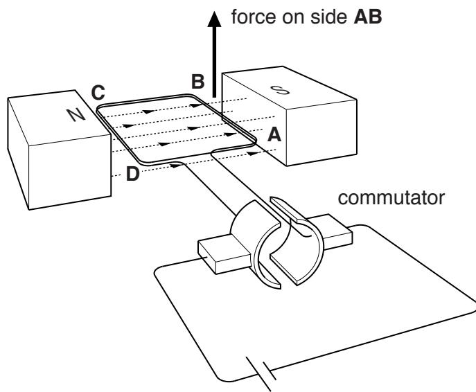
(a) The arrow on the diagram shows the force acting on side **AB** when a current flows in the coil.
