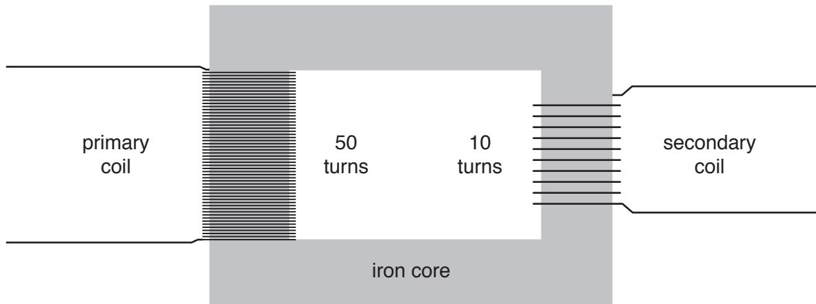
(a) A voltage is produced across the secondary coil when an alternating voltage is put across the primary.
