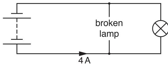
Callum's friend, Noah, says that when the broken lamp is replaced the 4A current will be shared between the two lamps, so each gets 2A. The total current from the battery will still be 4A. (You may assume that the lamps are alike.)
