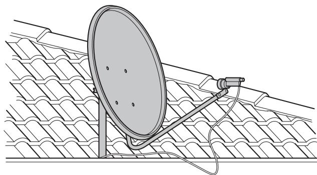
(a) A dish on the roof of a house guides the microwaves onto a receiver.
