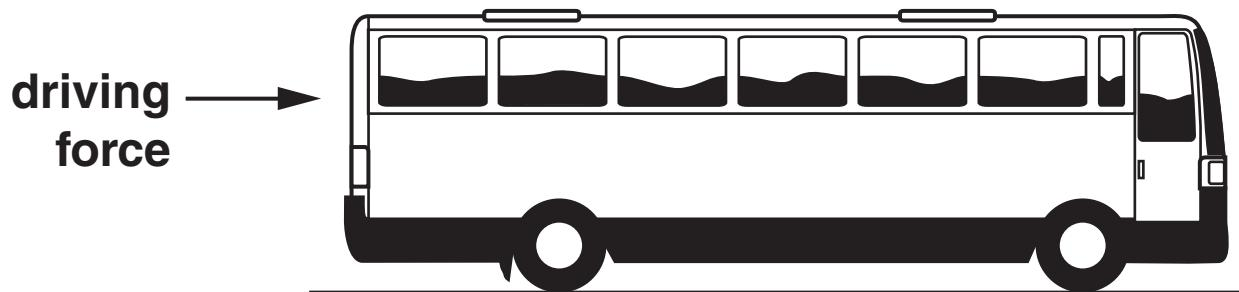
(a) A driving force acts forwards on the bus when it is moving at a steady speed.
