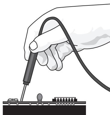
He needs to be careful. The chips in the circuit are easily damaged by static electricity.
