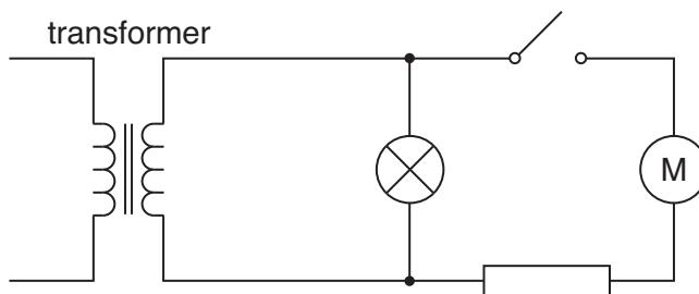
The circuit includes a switch to turn on the motor in the toothbrush.
