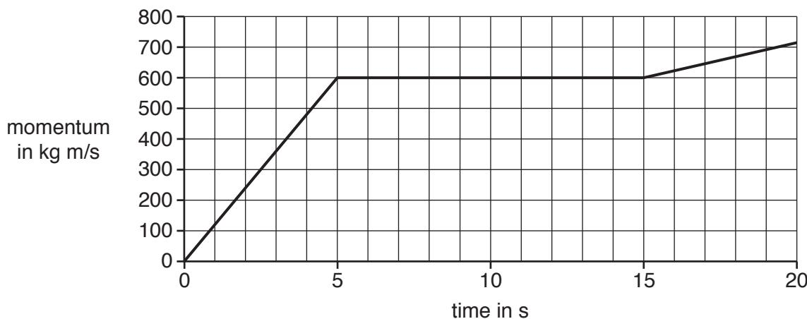
(i) Use data from the graph to calculate the resultant force acting on the wheelchair and the athlete during the first 5 seconds of the race.
