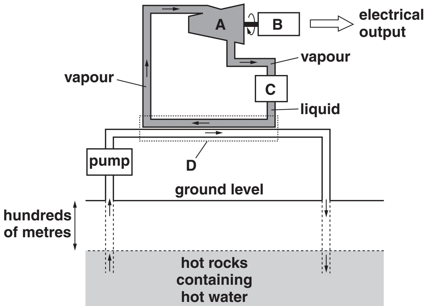
(a) The four parts A, B, C and D in the diagram are a CONDENSER, a GENERATOR, a HEAT EXCHANGER and a TURBINE.
