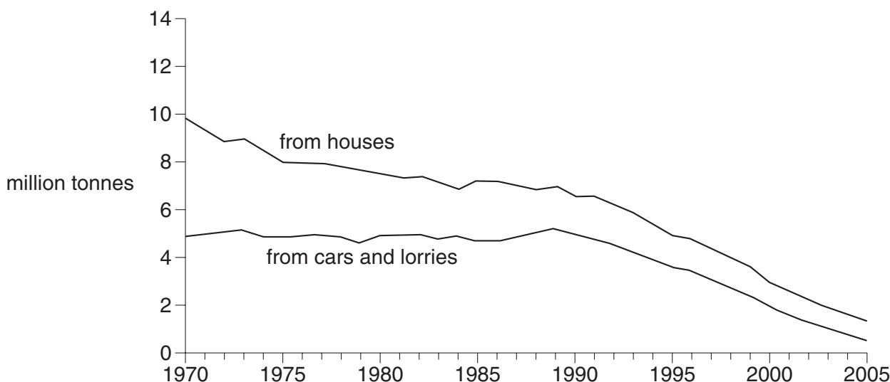
One way of removing carbon monoxide from car and lorry exhaust fumes is to use a **catalytic converter** (CAT). From 1989 onwards, more and more cars have been made with catalytic converters.
