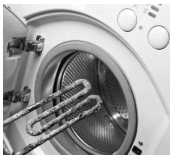
Lactic acid reacts with limescale and removes it from a heating element.
