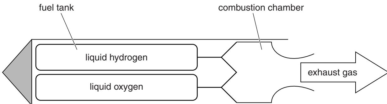
The hydrogen particles react violently with the oxygen particles in the combustion chamber.
