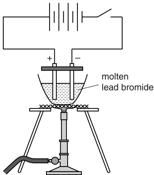
(a) **Solid** lead bromide cannot be electrolysed but **molten** lead bromide can be electrolysed.
