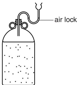
An air lock in the top of the jar allows gases to leave but stops air entering the jar.
