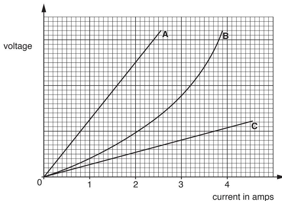
(i) Explain which component **A**, **B** or **C** has the highest resistance at 2A.
