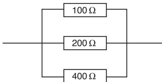
Calculate the **total** resistance of the three resistors in parallel.
