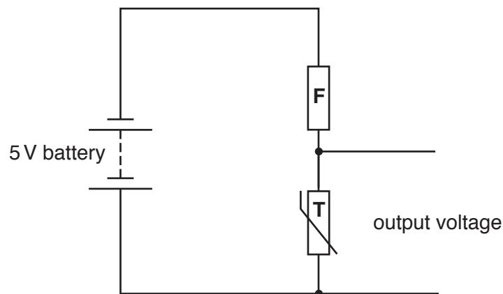
(a) The output of this circuit can provide a signal to a logic gate which depends on temperature.
