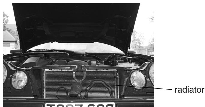
Hot water from the engine gives out heat in the radiator to keep the engine cool.
