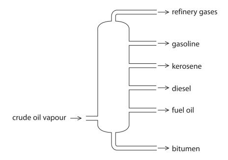
(i) Name the industrial process used to separate crude oil.
