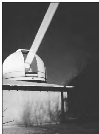
Laser light being sent to the Moon from a telescope in Germany.
