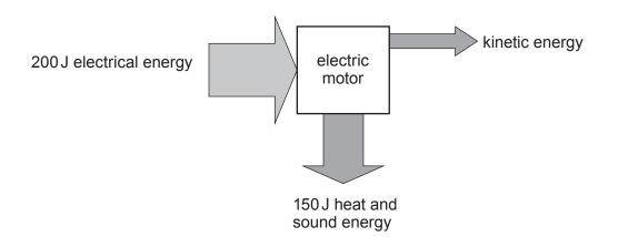
(i) Calculate how much useful energy the motor produces. [1]
